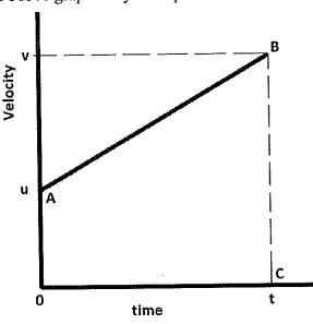
Ans: Alongside we have a velocity time graph of a body moving with constant acceleration. We know that the Displacement (S) = Area under the curve = Area of trapezium OABC =  $\frac{1}{2}$  x(OA + BC) x OC
