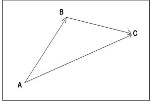
• **Parallelogram law** – If two vectors acting simultaneously at a point can be represented both in magnitude and direction by the two adjacent sides of a parallelogram, then their resultant is represented completely both in magnitude and direction by the diagonal of the parallelogram drawn from that point.
