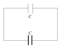
Ans. When two capacitors are connected to each other as shown in the figure, they have common potential V. Now charge on each capacitor, Q' = CV'.
