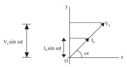
This diagram shows that the phase difference between I and V is zero
