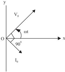
The phasor diagram for purely inductive circuit is shown in figure
