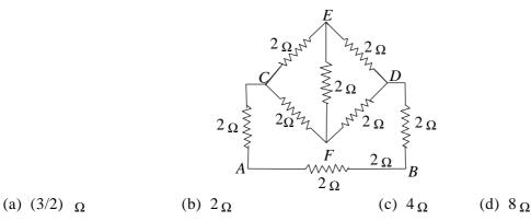
3. If each of the resistance in the network in figure is R, the equivalent resistance between terminals A and B is
