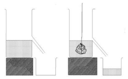
The volume of water overflows into a beaker is equal to the volume of solid Mass of solid =  $m_0$  g Mass of beaker and water= $m_2$  g Mass of beaker= $m_1g$ . Mass of water only =  $(m_2-m_1)g$
