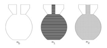
Mass of liquid=  $(m_1-m_0)g$ Mass of equal volume of water=  $(m_2-m_0)g$ Relative density= $\frac{mass of any volume of substance}{mass of an equal volume of water}$
