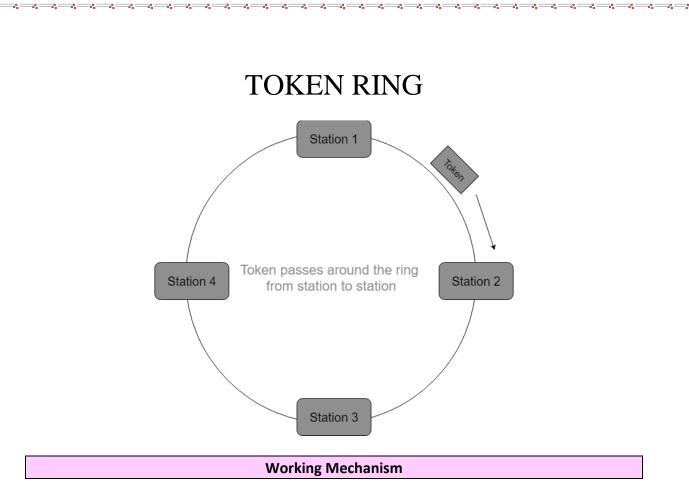
1. Systems in the LAN are arranged in a logical ring; each system receives data frames from its logical predecessor on the ring and sends them to its logical successor. The network may be an actual ring, with cabling connecting each node directly to its neighbours, but more often is a star, with the ring existing only logically in the wiring closet within the "multi-access unit" to which all the hosts connect.
